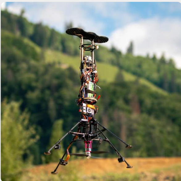
Test Platform for Colibri's GNC (Guidance, Navigation, and Control) System
