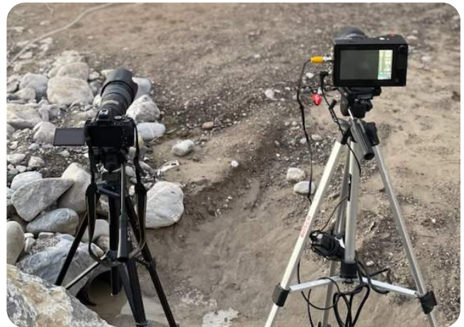
Behind-the-Scenes: Chronos 2.1-HD high-speed camera alongside a standard camera. This setup allows for the capture of both slow-motion footage and regular FPS filming.
